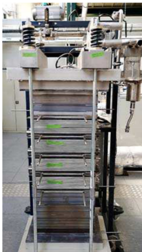
Figure 2: Assembled Integrated Modul for the 10/40 kW rSOC system without its thermal insulation (22).
